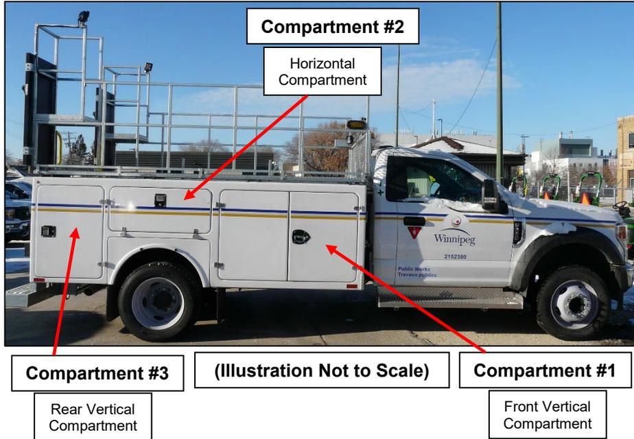
The present configuration of the service body compartment. (Passenger's Side – R1)
