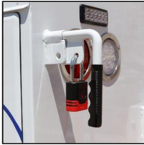
Representative Picture of Master Lock System for Aluminum Service Body.
