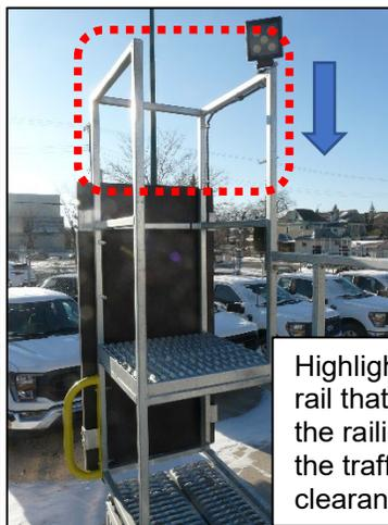
Highlighted in red is the portion of the rail that required collapsing/sliding into the railing tubing below to fit flush with the traffic advisor signal sign for clearance height areas.
