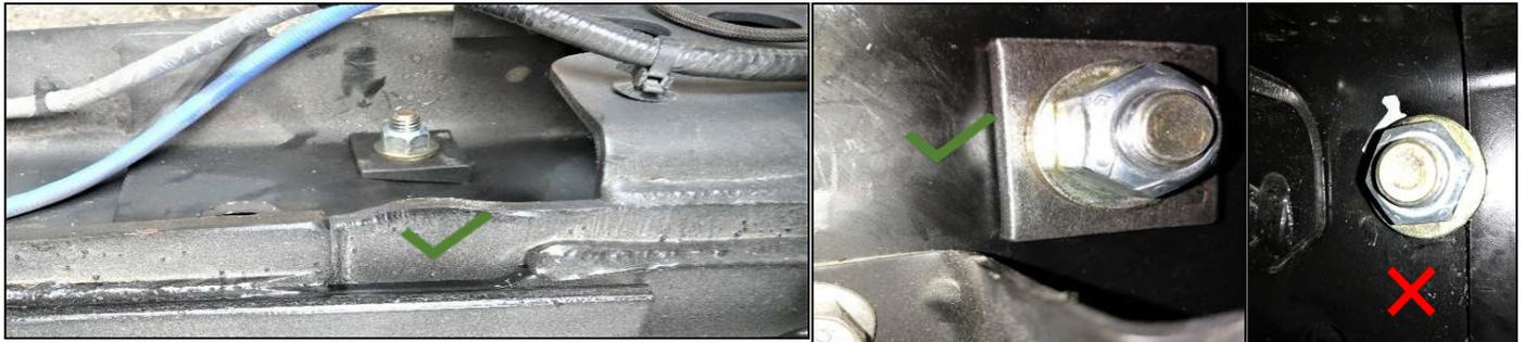
The assembly of bolt and nut through the chassis frame must adhere to certain guidelines. In the event that the hole is situated on a curved surface or where a transition occurs in the frame, it is not recommended to utilize it as a mounting location.
